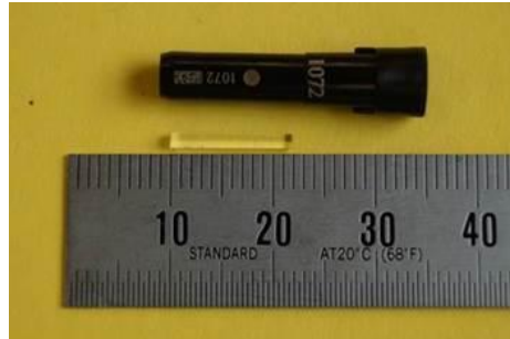
Fig. 3. RPLD: a protective plastic capsule with ID number and the glass rod.
